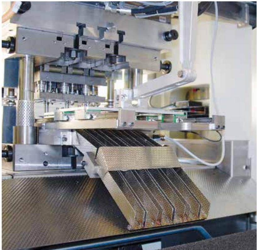
The removal device is integrated into the press control system to ensure damage-free part evacuation
