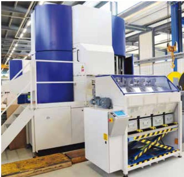
Carousel for separate multiple parts removal
