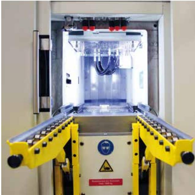
The die space in the XFT 1500speed is compatible with its GKP-100 and GKP-160 predecessors.
