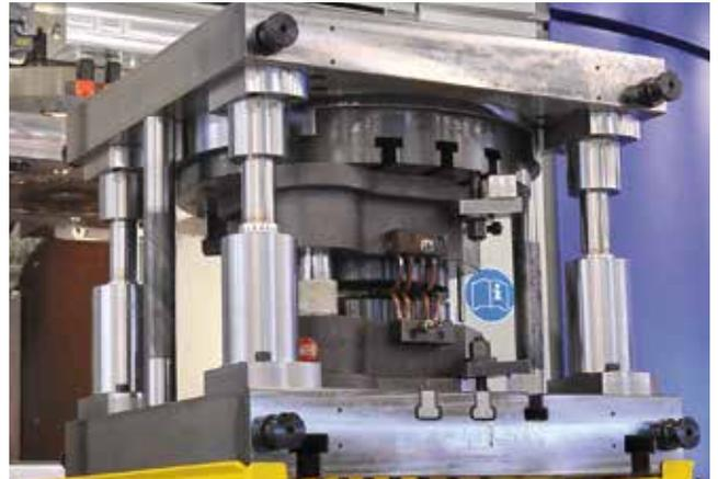
Thanks to the special adapter, the press does not need to be converted to use moving-punch tools.
