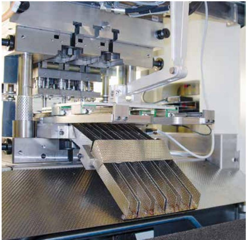
The removal device that is integrated into the press control system ensures that parts are removed undamaged and sorted by cavity
